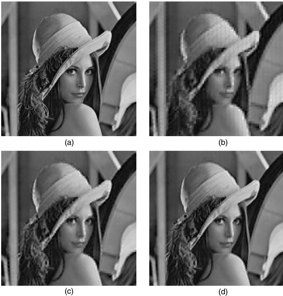
8.11 (a) The original “Lenna” image. Compressed “Lenna” using PCs obtained from the APEX model; (b) 4 PCs; (c) 8 PCs; and (d) 12 PCs. (Reproduced by special permission of Playboy Magazine. Copyright 1972, 2000.)
